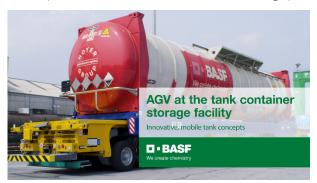
The transport from the tank container storage facility to the plants is carried out by an autonomous transport vehicle. The technical term is Automated Guided Vehicle or AGV for short. It can drive on normal roads — autonomously or automatically. The vehicle is electronically connected to a transponder lane and thus finds its way with centimeter precision.
