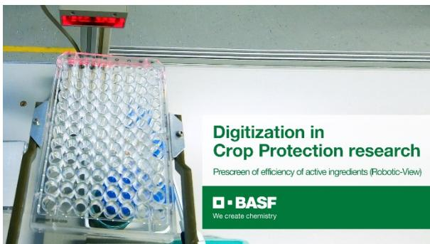
In the following step, copies – so-called daughter plates – are produced from the mother plates (microtiter plates) for each fungal disease, also in a fully automated process, and inoculated with the spores of the fungal pathogens. Up to 100,000 substances can be tested each year.
