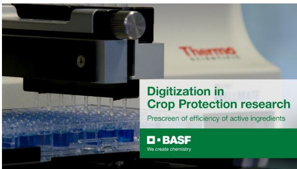
Prescreening is a procedure for the fully automated testing of active ingredients to determine biological effects. In this way, promising substances can be filtered out from a pool of substances.
