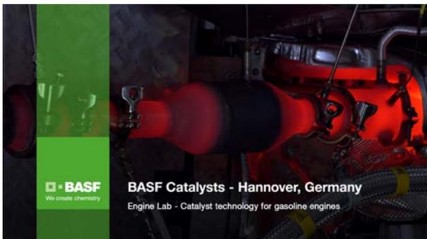
**Engine test bed for light duty cars with gasoline engine: The Technician installs a catalyst at the engine test bed right before the exhaust test. In the Hannover Engine Lab future catalyst technologies are tested on their functionality and durability under real life conditions.**
