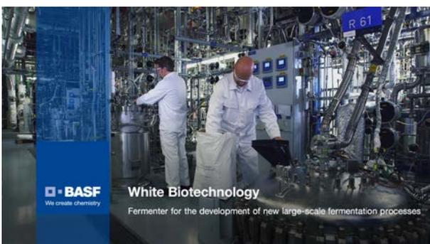
**Monitoring of the progress of fermentation in a 5000-liter fermenter in the biotech pilot plant.**
